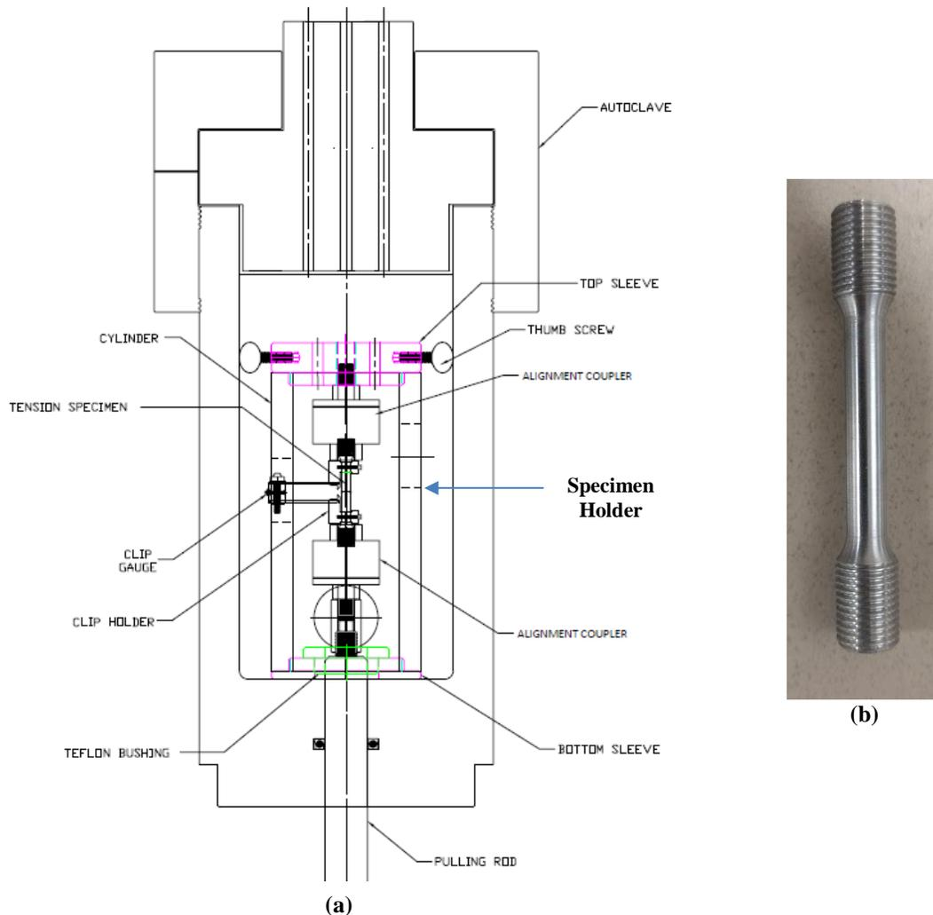
**Fig. 10. Assembly design of tensile test specimen with holder in autoclave (a) and photo of tensile specimen (b)**
