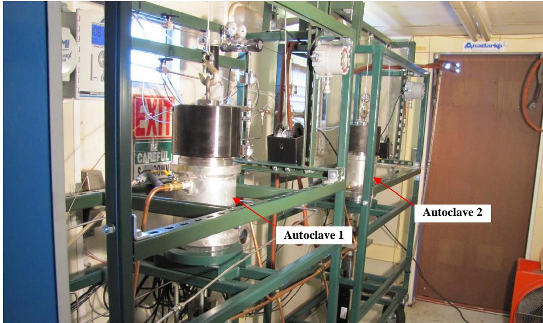
**Fig. 9: Experimental setups for testing hydrogen embrittlement**
