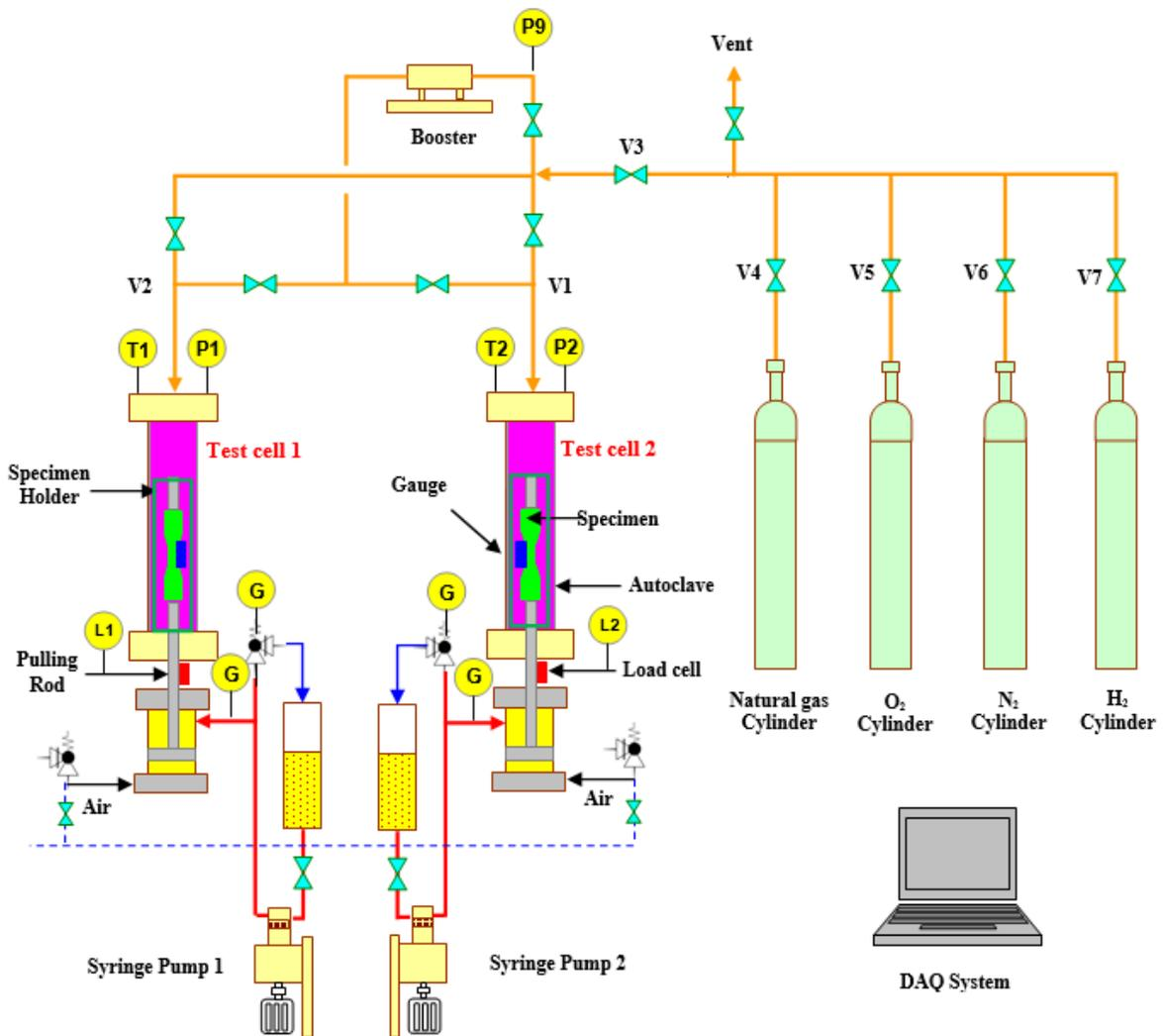
**Fig. 3: Simplified schematic of test setup**
