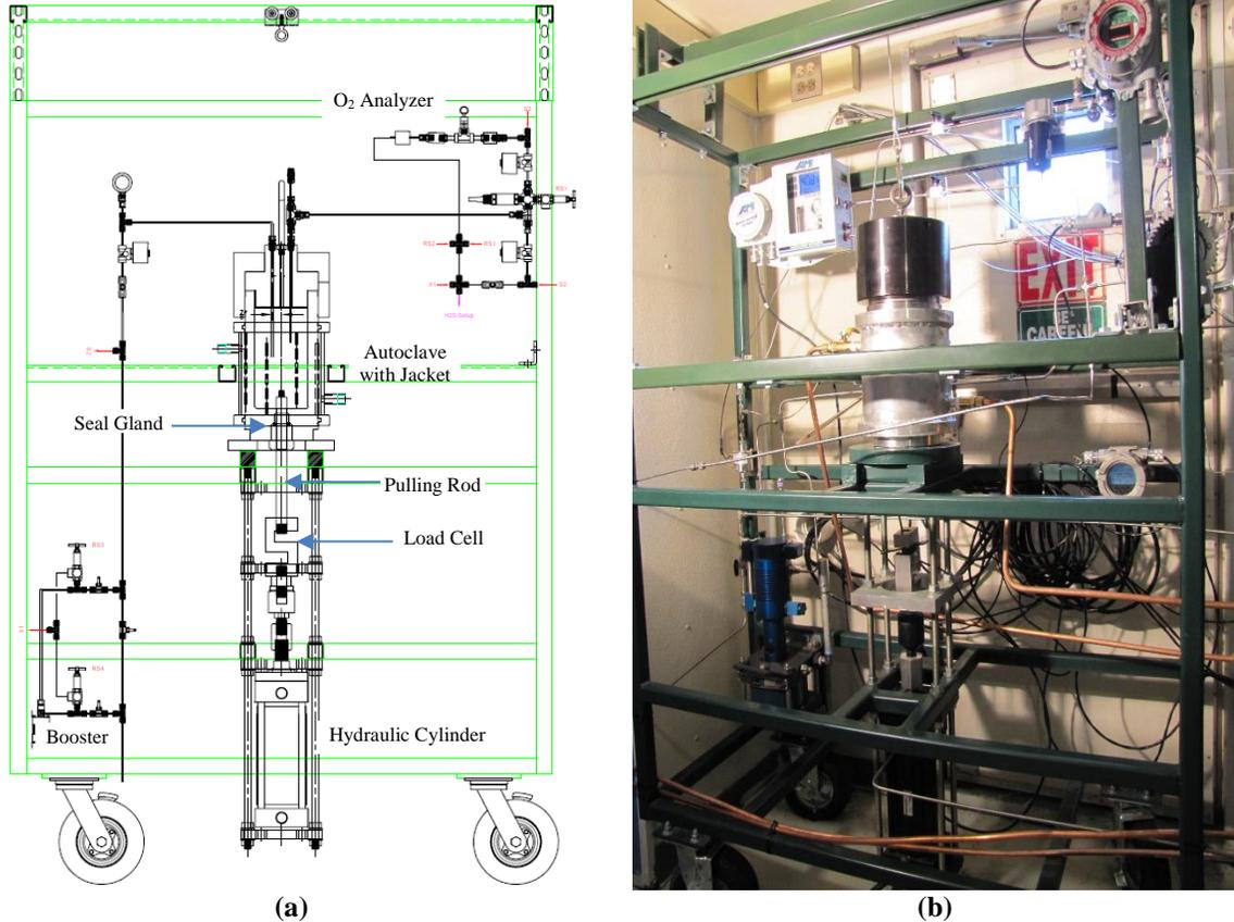
Fig. 7: Design (a) and photo (b) of experimental setup
