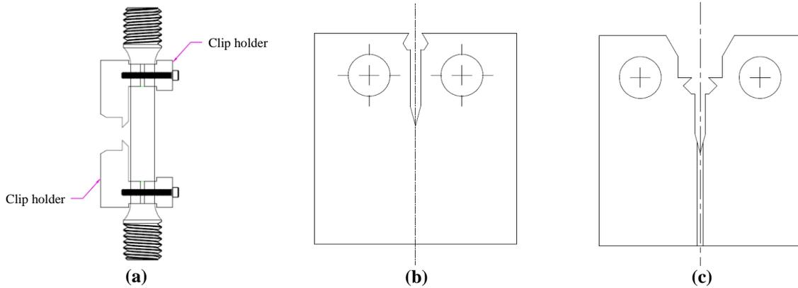
**Fig. 4: Specimen designs for different studies: a) tensile test; a) fatigue experiment; and c) fracture toughness test**
