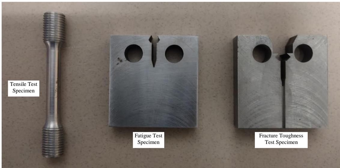
**Fig. 2: Test specimens cut from vintage pipes**
