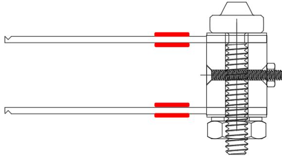
**Fig. 6: Custom-built clip gauge**
