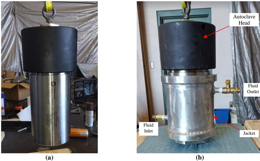
**Fig. 5: Autoclave before (a) and after (b) covered with a heating jacket**
